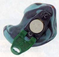
Left: The active package is removable and can be replaced with passive inserts
